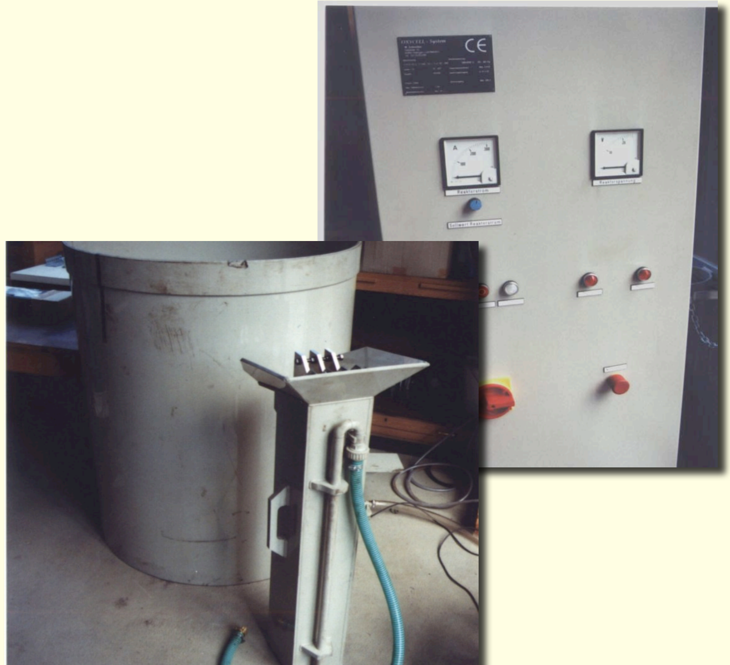
Process Unit with Reactor Volume of 30 L
